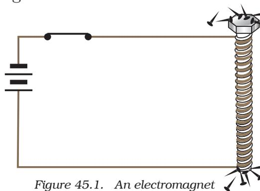
Figure 45.1. An electromagnet
