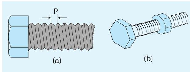
**Fig.E 2.1** A screw (a) without nut (b) with nut
