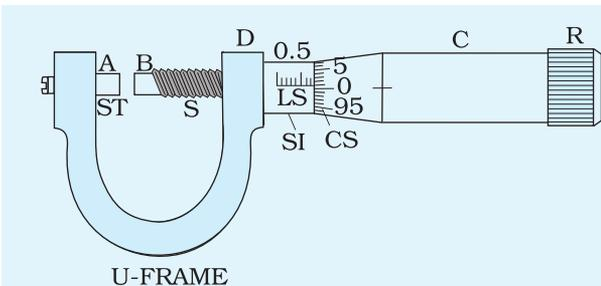
**Fig.E 2.2:** View of a screw gauge
