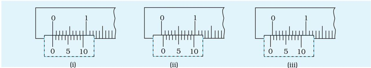
**Fig. E 1.2:** Zero error (i) no zero error (ii) positive zero error
