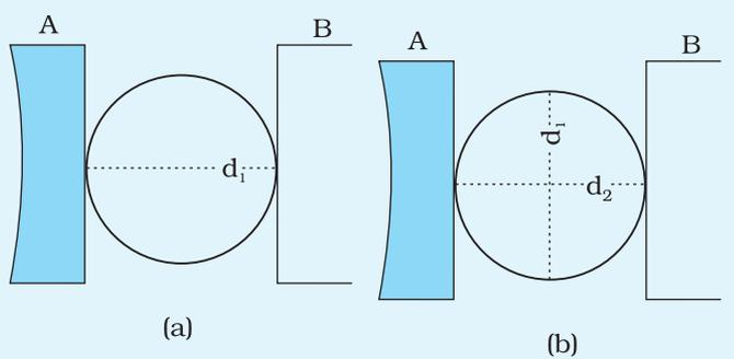
**Fig.E 2.6 (a):** Two magnified views (a) and (b) of a wire showing its perpendicular diameters  $d_1$  and  $d_2$ .  $d_2$  is obtained after the rotating the wire in the clockwise direction through  $90^\circ$ .
