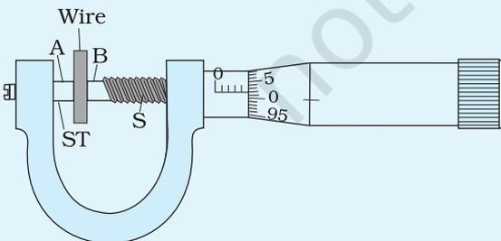
**Fig.E 2.5:** Measuring thickness with a screw gauge
