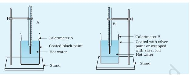
**Fig. P 10.1(a):** Experimental setup for studying emission of heat radiation from black surface
