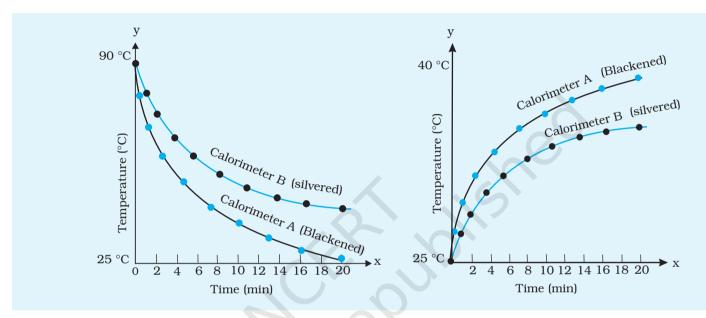
**Fig. P 10.2(a):** Temperature vs. time graph for **Fig. P 10.2(b):** Temperature vs. time graph for emission of heat radiation absorption of heat radiation
