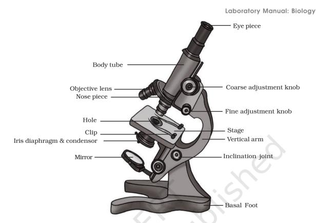
Fig.1.1 A compound microscope
