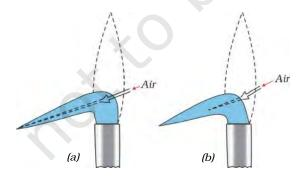
Fig. 7.7: Obtaining oxidising and reducing flame (a) Oxidising flame; and (b) Reducing flame
