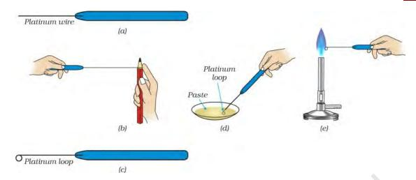
Fig. 7.3: Performing flame test
