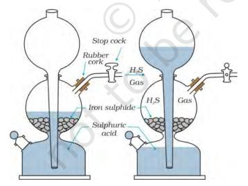
Fig. 7.8: Kipp's apparatus for preparation of  $H_2S$  gas
