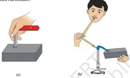
Fig. 7.6: (a) Making charcoal cavity (b) Heating salt in the cavity
